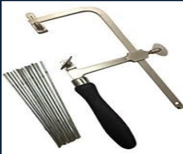
15. Jewelers Saw with multiple blades or blade kit. Essential for cutting material with the ability to turn tight corners or shapes.
